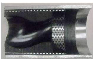
Fig. 7. Detail of reinforcement of chemical bonding by using stainless steel net welded to the stator tube
