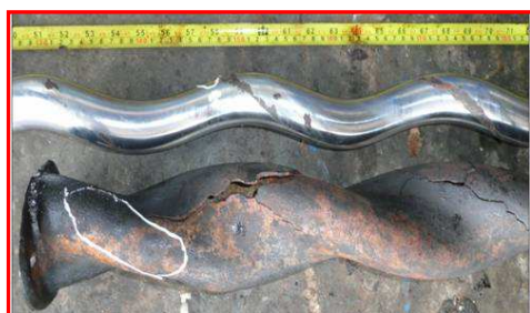
Fig. 6. Discharge section of the all metal PCP that failed in the well MFB-722
